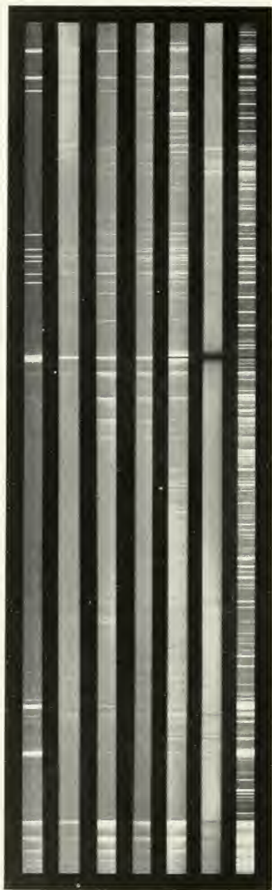
THE SPECTRUM OF CALCIUM IN THE ARC AND IN THE ELECTRIC FURNACE, SHOWING THE EFFECTS OF CHANGING THE TEMPERATURE AND THE QUANTITY OF VAPOR
